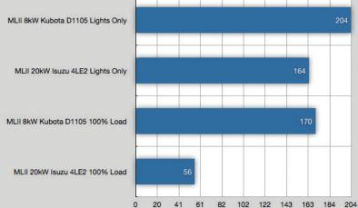
Run Time on One Tank of Fuel (Hours)
